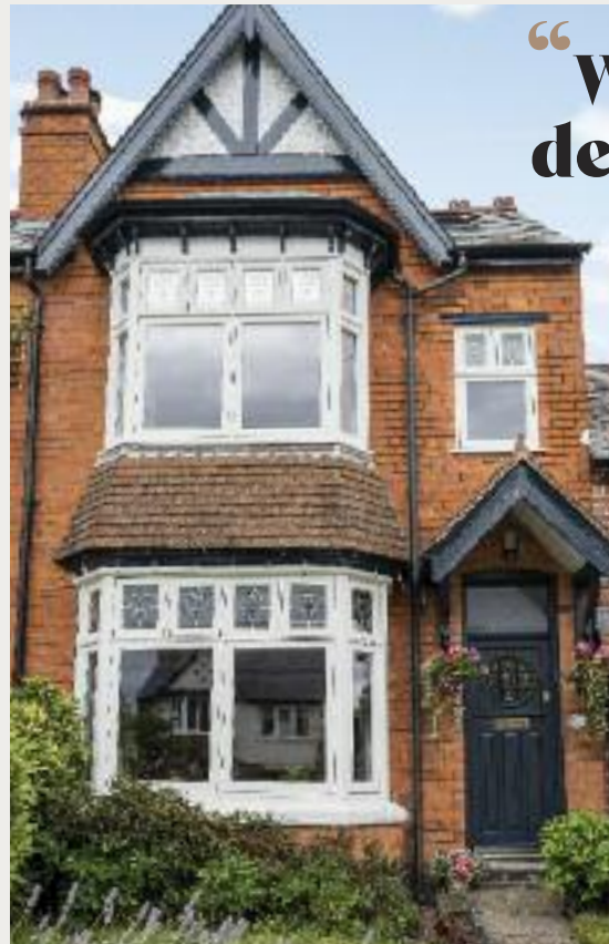
Deco casement windows finished in 'Off-White' with a bespoke, signature stained glass design and manufactured in Engineered European Redwood.
