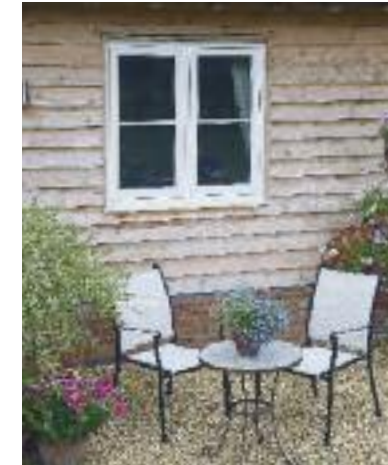
Flush casement windows finished in 'Off-White' with large Pewter Monkeytail handles and pegstays, and 18mm astragal glazing bars.
